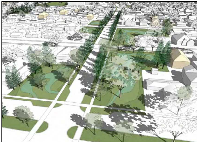
View of Corner Street Basins and Storm water Lots at Mirabeau Image printed with permission and courtesy of NORA.
