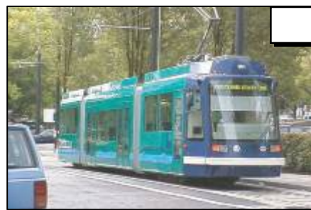
Streetcar • Steel wheel on rail • Rail right-of-way that can be exclusive or in mixed traffic along city streets • Often 1 vehicle but can consist of more than 1 vehicles connected • Low (10-25 mph), depends on number of stops
