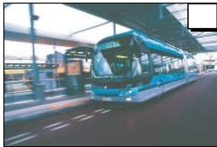
Bus Rapid Transit (BRT) • Rubber tire on pavement • Exclusive road right-of-way or mixed traffic on city streets • Can be 1 vehicle or more than 1 vehicle connected • Medium (30-50 mph)
