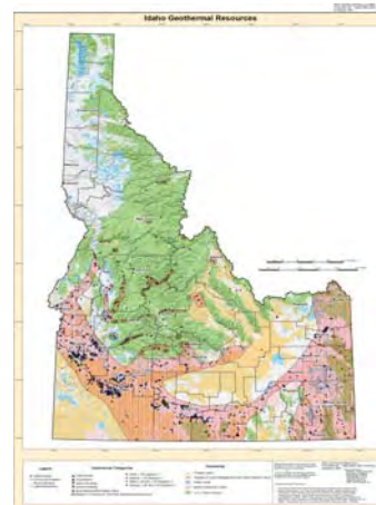
Geothermal Resources- Pink indicates areas of known or potential geothermal resources.
